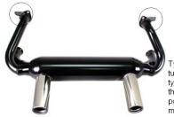
Typical header system with heat riser tube flanges but not a bypass tube. This type of exhaust will have very poor flow through the heat riser tube and very poor intake manifold heat without the modification described.
