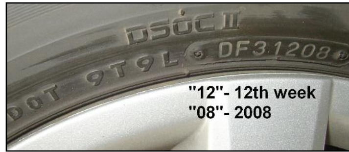
This tire is on my wife's car, bought a couple of years ago. The tire was made in the 12th week of 2008
