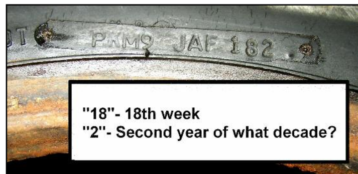
This tire was on a junk vehicle that has not moved in at least 15-20 years. We know it was made in the 18th week of the 2nd year of the decade, but which decade? It could be May of 1992, or May of 1982, we'll never know. This tire was severely dry rotted, leaking through the sidewall, and "checking cracks" can be seen in the photo.
